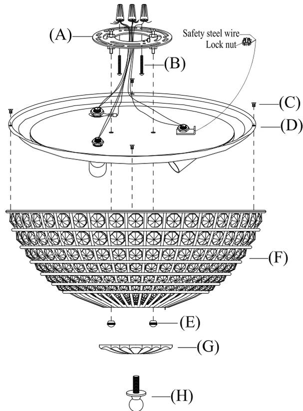
1. Remove mounting plate (A) from fixture base (D) by unscrewing cap nuts (E).
